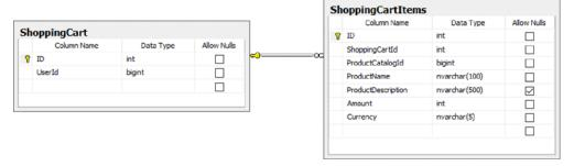
Figure 5.6 ShoppingCart has only two tables: one has a row for each shopping cart, and the other has a row per item in a shopping cart.
