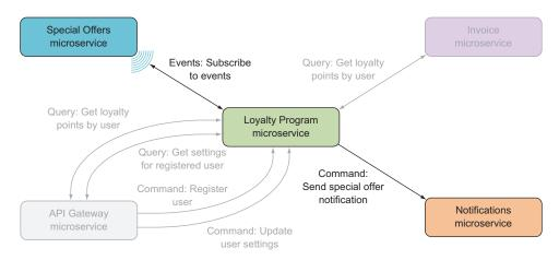
Figure 4.12 The event-based collaboration in the Loyalty Program microservice is the subscription to the event feed in the Special Offers microservice.
