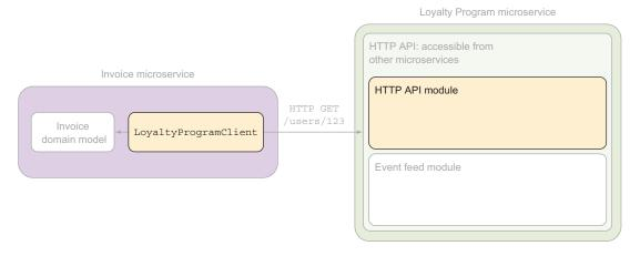
Figure 4.6 The LoyaltyProgramClient component in the Invoice microservice is responsible for making calls to the Loyalty Program microservice. It translates between the contract published by Loyalty Program and the domain model of Invoice.
