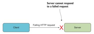
Figure 6.4 All collaborations between microservices have a client and a server. The client sends HTTP requests to the server. The client is responsible for handling failed requests.
