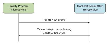
Figure 7.3 For service-level testing, the Loyalty Program microservice interacts with mocked versions of its collaborators. The mocked microservices respond to requests with hardcoded responses.
