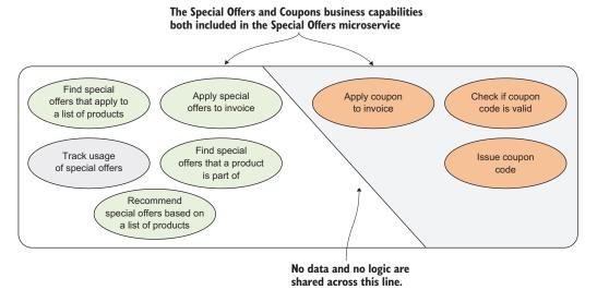
Figure 3.12 If you choose to err on the side of bigger scopes, you might decide to include the handling of coupons in the Special Offers business capability.
