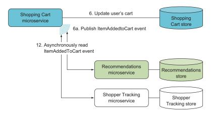
Figure 2.9 The Shopping Cart microservice publishes events about changes to shopping carts to an event feed. The Recommendations and Shopper Tracking microservices subscribe to these events and react as events arrive.
