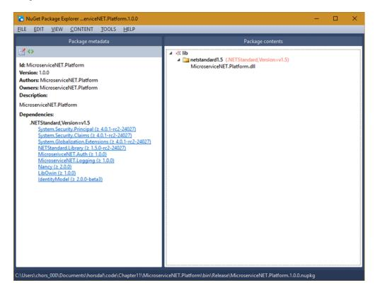
Figure 11.5 Looking in MicroserviceNET.Platform.1.0.0.nupkg shows that the package depends on the other two packages in the platform—MicroserviceNET.Logging and MicroserviceNET.Auth—as well as a number of external packages.
