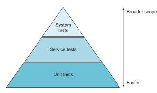
Figure 7.1 The test pyramid illustrates that you should have a few system-level tests, many service-level tests, and even more unit-level tests.
