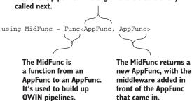
A function that takes in an AppFunc returns another AppFunc. A MidFunc is a function that takes in an AppFunc implementing an OWIN pipeline consisting of zero or more pieces of OWIN middleware, adds a piece of middleware in front of that, and returns an AppFunc for the new pipeline.
