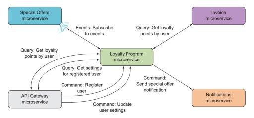
Figure 7.2 The Loyalty Program microservice collaborates with a number of other microservices through all three types of collaboration: events, queries, and commands.
