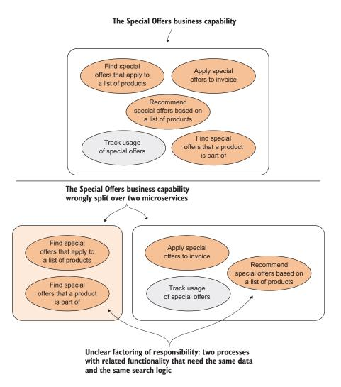
Figure 3.11 If you make the scope of a microservice too small, you'll find that a single business capability becomes split over several highly coupled parts.
