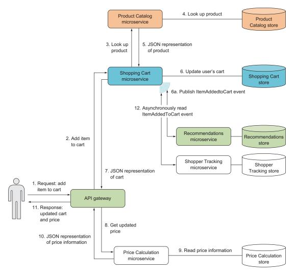
Figure 2.1 The Shopping Cart microservice allows other microservices to get a shopping cart, add items to and delete items from a shopping cart, and subscribe to events from Shopping Cart.
