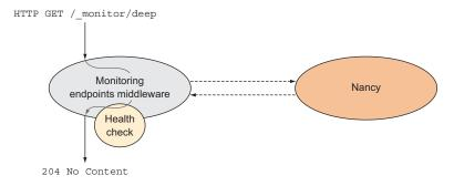
Figure 9.4 You can put monitoring endpoints in a piece of OWIN middleware in front of Nancy. When a request to the /\_monitor/shallow endpoint comes in, the monitoring middleware gives a 204 No Content response. When a request to the /\_monitor/deep endpoint comes in, the monitoring middleware calls a function that performs a health check and then responds with 204 No Content if the health check succeeded. Other requests pass through the monitoring middleware and on to Nancy.
