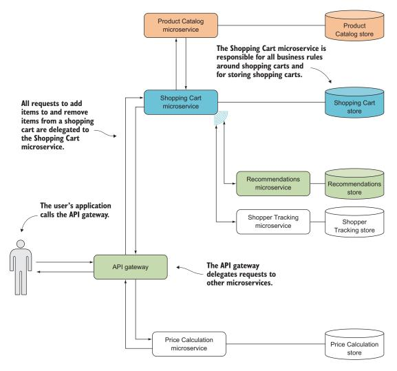
Figure 12.7 The Shopping Cart Microservice is responsible for storing and maintaining shopping carts on behalf of users, but the API gateway makes that functionality (along with other pieces of functionality) available to end users to use in a web app.
