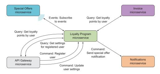
Figure 4.2 The Loyalty Program microservice uses all three collaboration styles: commands, queries, and events.
