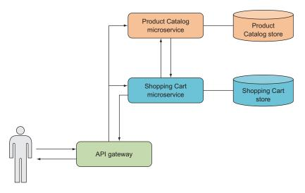
Figure 12.8 This example focuses on the API gateway, the Product Catalog microservice, and the Shopping Cart microservice. You'll implement part of an application based on those three.
