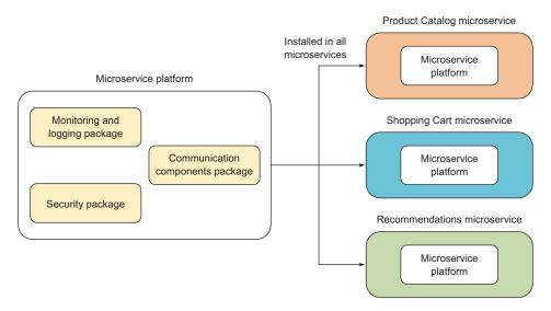
Figure 11.1 The microservice platform is a collection of packages implementing the technical concerns that cut across all microservices. The platform is installed in—and thus becomes part of—every microservice.
