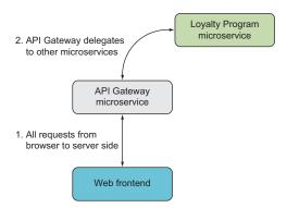
Figure 10.2 The web frontend for users of the loyalty program communicates only with the API gateway.
