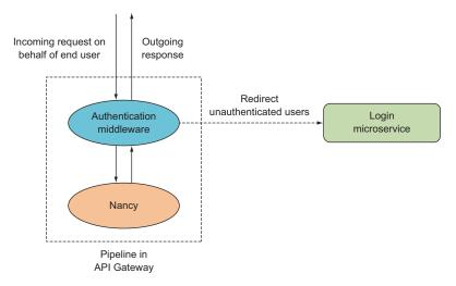
Figure 10.5 Use authentication middleware to redirect unauthenticated users to the Login microservice.
