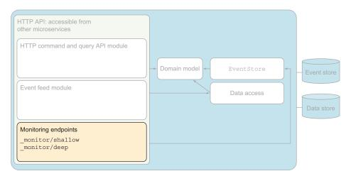
Figure 9.3 Every microservice should have two monitoring endpoints: one at /\_monitor/shallow and one at /\_monitor/deep. The monitoring system polls both endpoints. As long as both respond with a success response, the monitor considers the microservice to be up.
