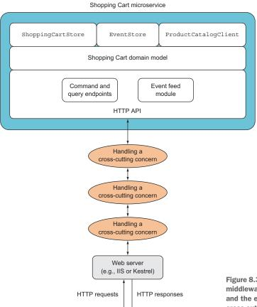
Figure 8.3 You can use a pipeline of middleware between the web server and the endpoint handler to handle cross-cutting concerns.
